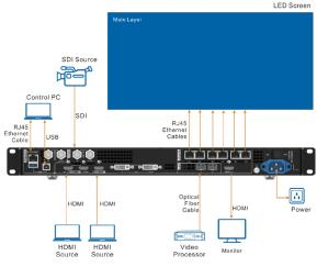
The processor does not present a controllable display to the MediaMaster System, only a video output for an MM-127x or MM-177x series decoder. This gives you audio control via the optional line-level output, but to control the display's power, you will require additional hardware. Consult ETR for details.
